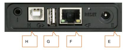
Those connectors are behind a trapdoor. It must remain close in industrial environment to preserve the IP65 protection. Use those connectors only in office environment.
