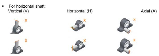
For horizontal shaft and Axial (A), Radial oblique 1 (1) and Radial oblique 2 (2) directions
